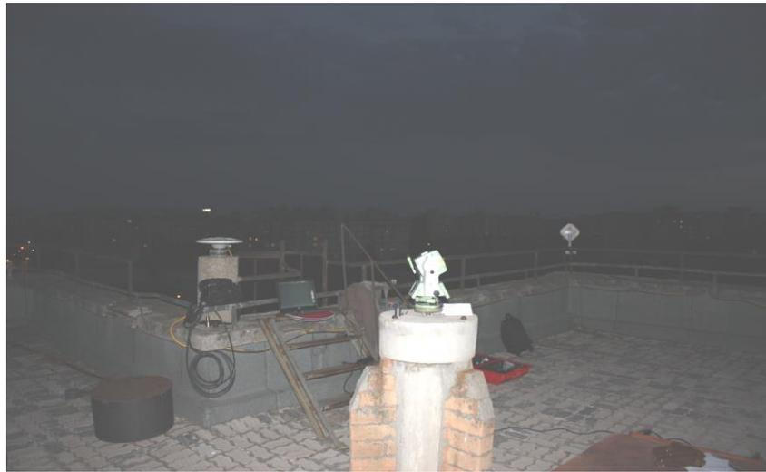
Fig. 5. Pilaster on the roof of BTUCE Faculty of Geodesy, and Leica TCRP 1201+ during astro-geodetic determinations (year 2012).
